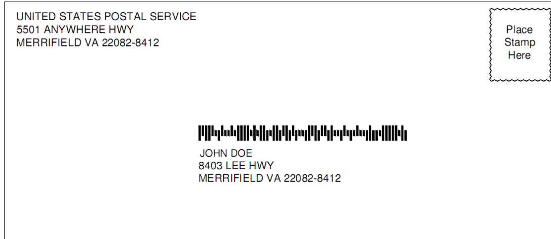
Figure 7: Intelligent Mail Bar Codes – 4-state bar code
